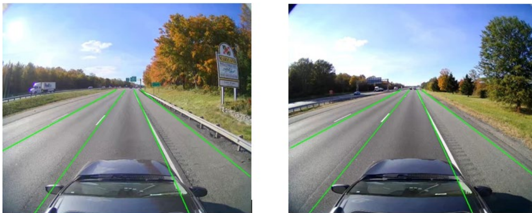
Figure 11. Image overlay. The images show the application of the CLRRerNET algorithm to ADS CONOPS Cross-Country data to measure shoulder width.
