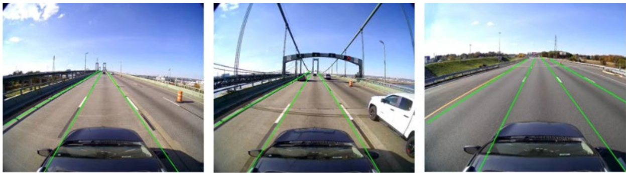
Figure 12. Image overlay. The images show the application of the CLRerNET algorithm to ADS CONOPS Cross-Country data to measure lane lines.
